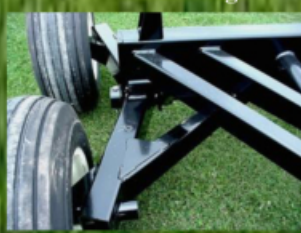
WishBoneType Tandem Axles On All Wagons
