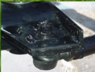
Ball Joint Steering On All Wagons
